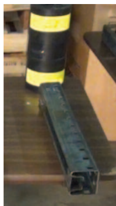
As shown above, the RAM Guard and 13 gage column were undamaged after 6 impacts. In fact, the same column and RAM Guard were tested an additional 14 times and remained fully functional!
