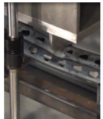
An unprotected 13 gage column after 2 impacts shows significant damage
