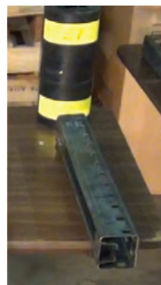
As shown above, the RAMGuard and 13 gage column were undamaged after 6 impacts. In fact, the same column and RAMGuard were tested an additional 14 times and remained fully functional!
